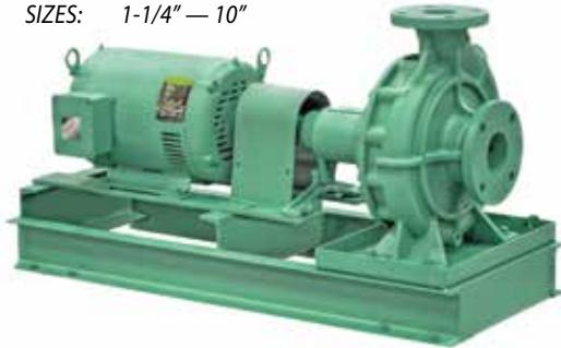
Cast iron casing with integrally cast feet enables pump to be bolted to base for sturdier installation. Allows for back pull without disturbing piping.
