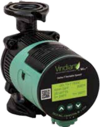
**Viridian® VT2218** circulator is a temperature sensing, self-adjusting, variable speed wet rotor circulator with an ECM permanent magnet motor. Operating modes include Delta-T differential temperature, 4 fixed speeds, set point heat, set point cool and boiler protection.
