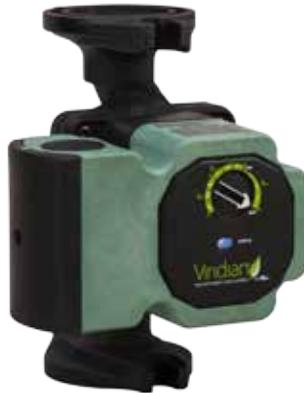
**Viridian® VR1816** circulator is an infinitely variable speed, high efficiency wet rotor circulator with an ECM permanent magnet motor. Operating modes include infinitely variable fixed speed and self-adjusting constant pressure or proportional pressure variable speed.
