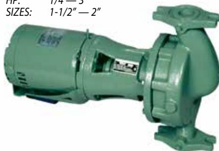
Rugged casing design has maximum operating pressure of 175 psi and a maximum operating temperature of 300°F. The 1600 Series is offered in cast iron stainless steel-fitted or all-stainless steel construction.
