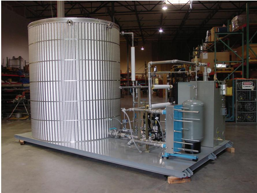
Proctor Sales Inc worked directly with the engineer to execute this package that is based on a Japanese design. This skid has two point mechanical and electrical connections for quick and easy site installation.
